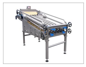
The principle of the mussel sorter is based on revolving rollers, provided with a spiral so that the mussels can be transported via this spiral 1 by 1. All rollers are driven by 1 motor, and the machine is adjustable from all angles.
